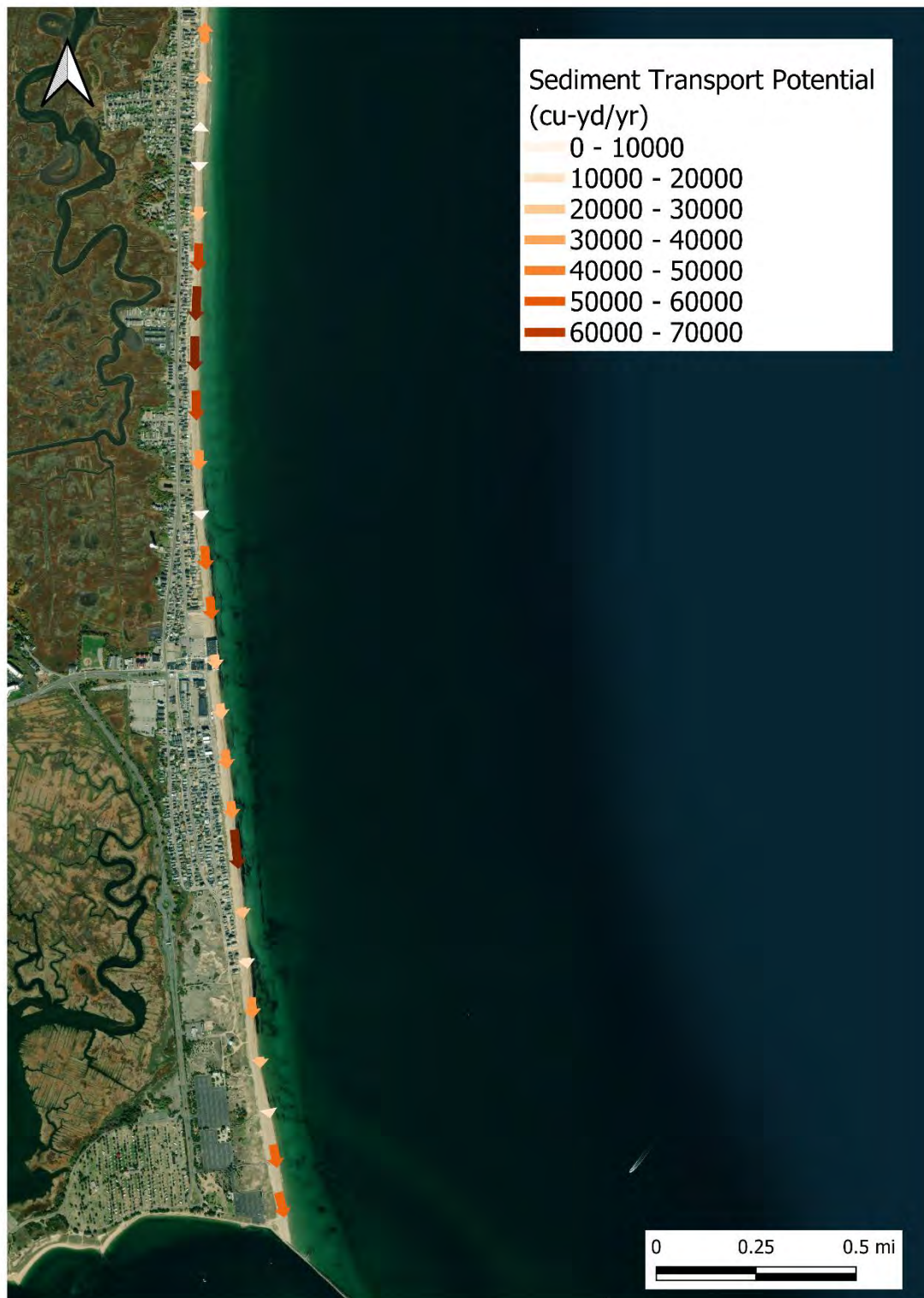
Figure 4.10. Computed net annual sediment transport potential rates along the Salisbury Beach shoreline. Arrows indicate the direction of transport, while the color and size of the arrows indicate transport magnitude.
