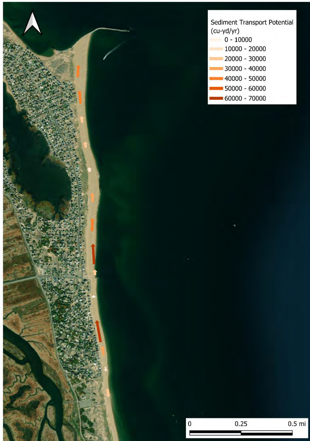
Figure 4.11. Computed net annual sediment transport potential rates along Plum Island Beach shoreline. Arrows indicate the direction of transport, while the color and size of the arrows indicate transport magnitude.
